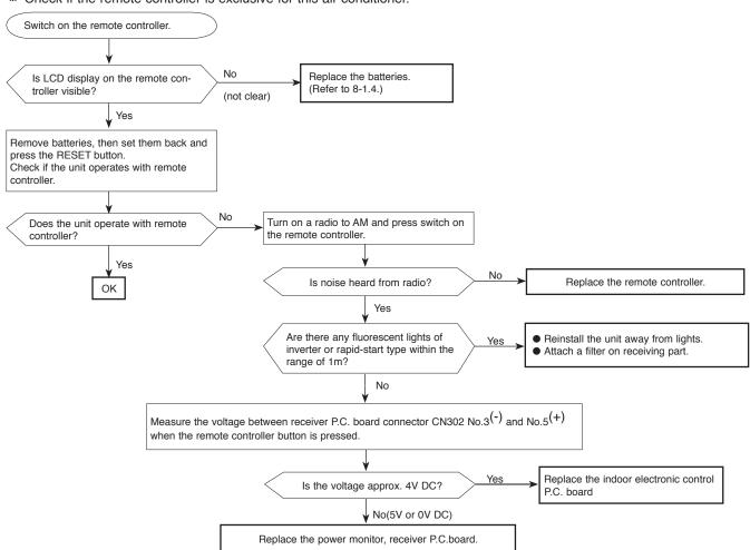
The unit doesn't operate with the remote controller.
